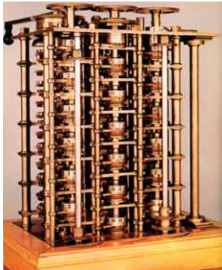
Figure-5: Charles Babbage Difference Engine
